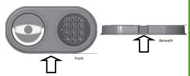
You'll find the battery compartment underneathe the electronic lock.
